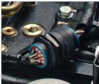
IP66 Sealed Connector
